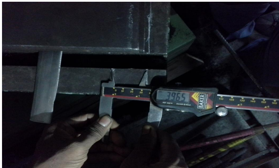
Figure 15: Deflection in the leaf spring
